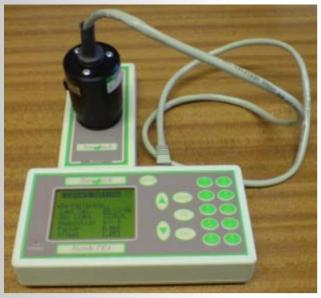
The LED array within the Handy PEA sensor head is focused, using lenses, down to a 4mm diameter measurement area. This coincides with the measurement area of the leafclips and ensures that the maximum possible intensity is delivered from the LED array directly onto the sample surface.
