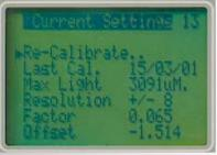
The light source calibration factor is calculated from a simple 2 point reading of a high and low light intensities. The calibration routine itself is accessed by selecting the Calibrate Light option from the Configure menu screen to display the information as shown in the opposite image. Selecting Re-Calibrate from this screen will initiate a fully automated calibration routine.
