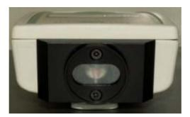
The Pocket PEA optical interface is mounted directly on to the front of the Pocket PEA control unit. It consists of a single high intensity focused LED which is positioned vertically above the sample. The light emitted from the LED is filtered using an NIR filter to block any infra red content which could be seen by the detector (this is known as optical breakthrough). The fluorescence detector is fitted with an RG9 filter to further eliminate the chance of optical breakthrough.
