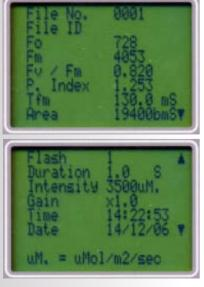
Press the down arrow key to display details of the measurement protocol use to take the measurement as shown in the following image.
