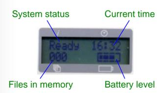
When in standby mode, the LCD display shows information regarding the current status of the Pocket PEA control unit as shown in the diagram above. Once a measurement is initiated, the LCD indicates that a recording is taking place and displays the illumination intensity. Fv/Fm and PI (Performance Index) parameter values are automatically calculated and displayed for 5 seconds once the measurement has completed before returning to standby mode.
