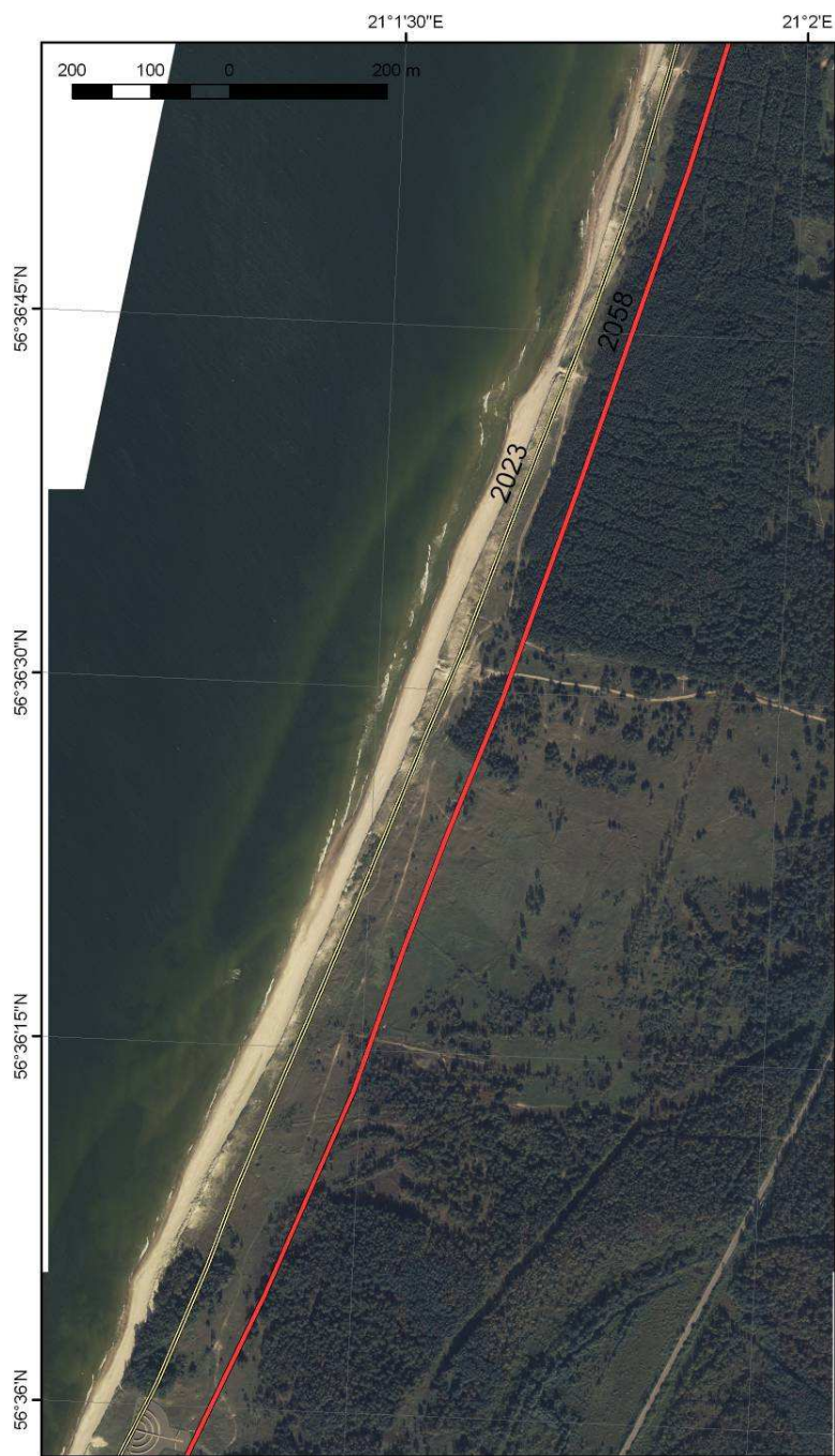
Fig. 4.1. Coastal erosion risk zone for 15 and 50 year period. Visualization of digital data layer, base – orthophoto from „Metrum” Ltd.
